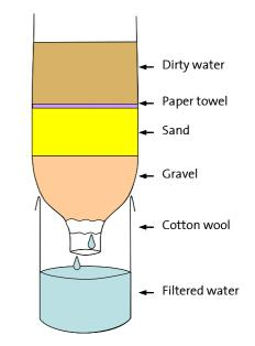
You have now constructed your filter and are nearly ready to test it. All you need to do is stand the filter (with the cotton wool at the bottom!) on top of the beaker.
