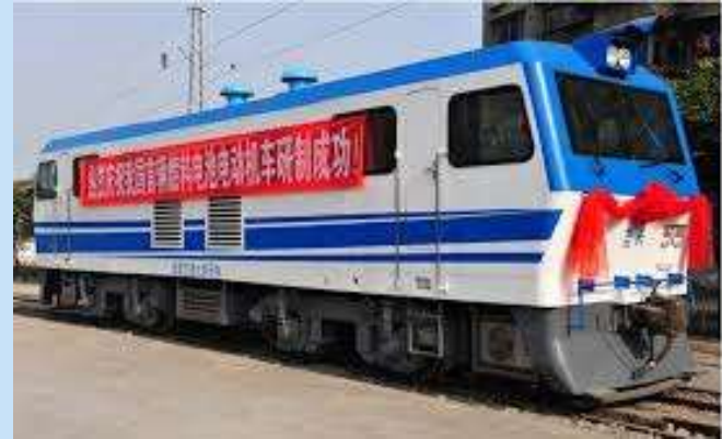
2013, China 45 tonne locomotive 150 kW fuel cell
