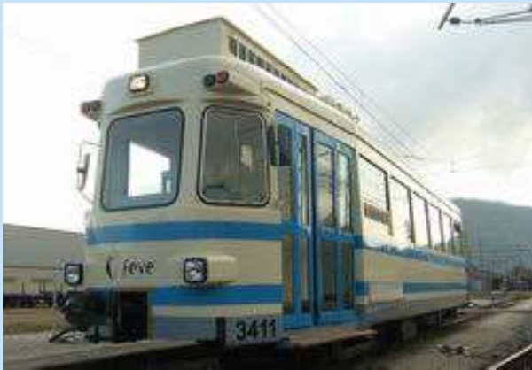
2011, Spain Metre-gauge tram 2 x 12 kW fuel cells
