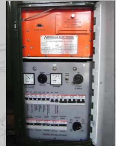
Auxiliary Services I/O Panel with OTMR above
