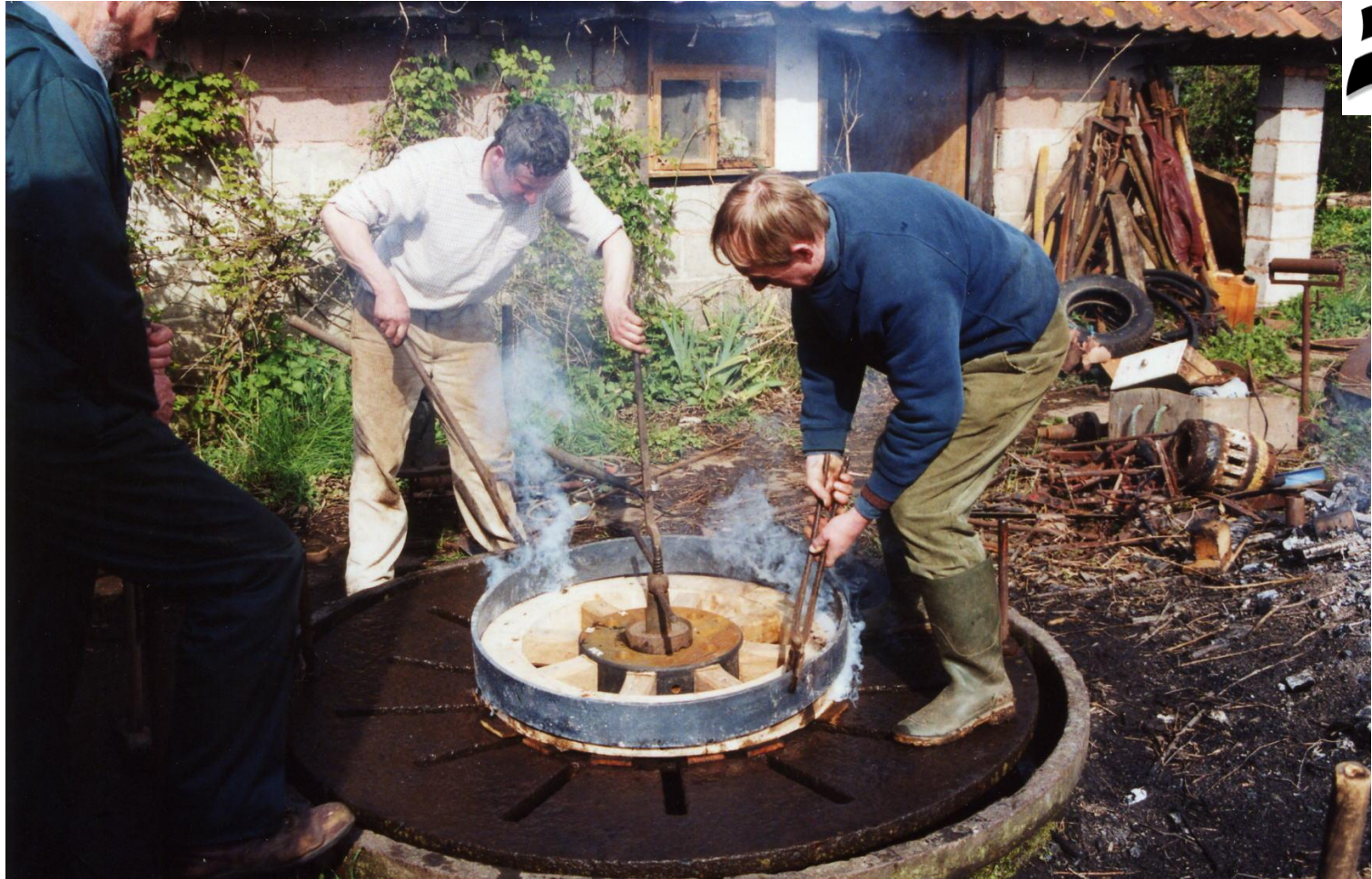
Placing the hot tyre on the wooden wheel
