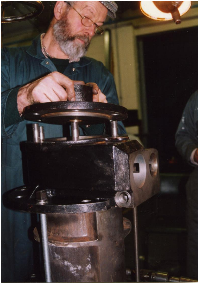
John Sawle assembling the cylinder head And the wax piston lubricator
