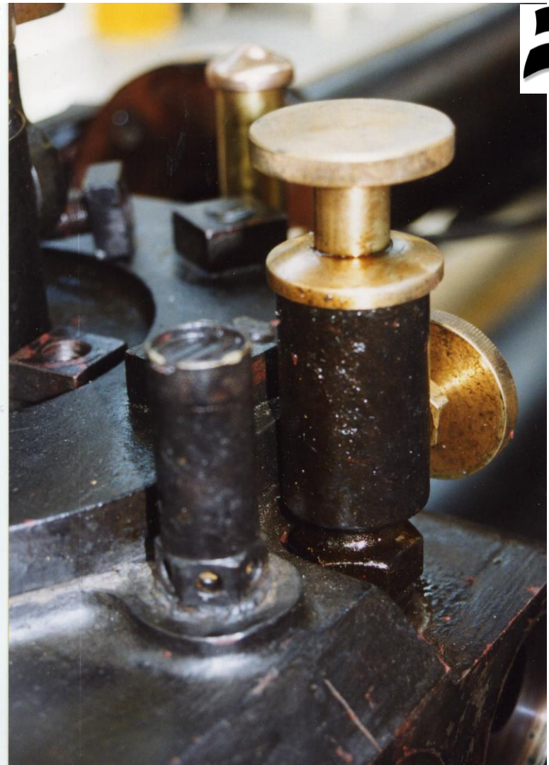
John Sawle assembling the cylinder head And the wax piston lubricator
