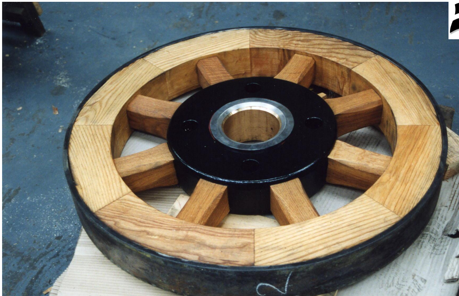
A completed wheel. Oak spokes and ash fellies. Weight 2 cwt
