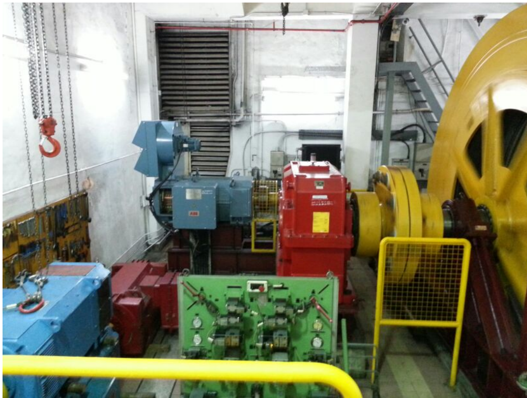
d.c. motor (blue, left), gearbox (red, middle), coupling (behind fence) and Haulage Drum (yellow far right) [W.H. Tsang]
