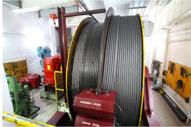
Emergency Brake (top) and Service Brake (bottom) apply brake on the brake flange on Haulage Drum [Benny C.Y. Sit]
