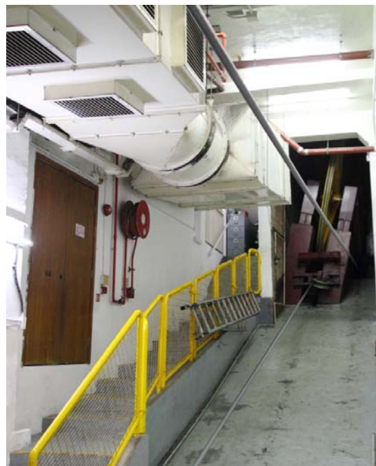
Deflection Sheaves offset the Hauling Ropes leaving the Haulage Room [Benny C.Y. Sit]
