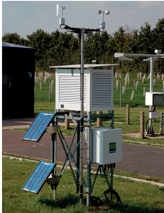
Figure 6. AA Stevenson screen and its surroundings. Met Office 2018c . (© Crown Copyright Met Office 2018)
