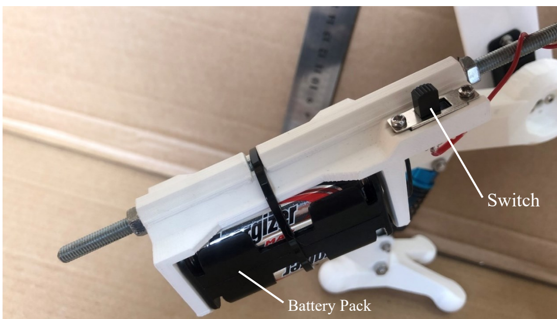
Figure 16: The “tail” of Pavo, housing the batteries and a power switch, both labelled
