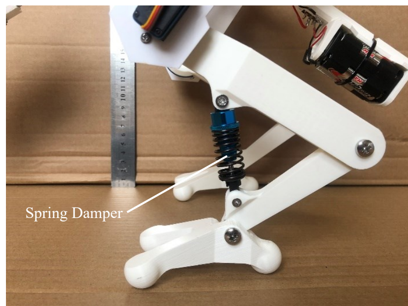
Figure 18: The left foot assembly of Pavo with spring damper labelled
