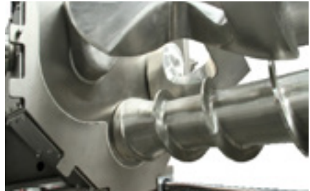
A Z-blade industrial mixer used for mixing, kneading and dispersion of very viscous doughs and pastes. This food quality machine is shown with the casing removed for cleaning.
