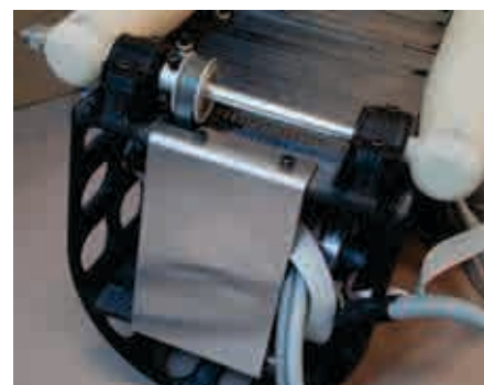
Photos of the finished robot (complete with realistic fur), the inner workings of the robot and the leg actuator mechanisms
