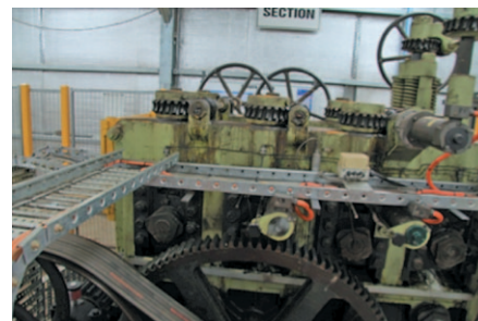
A beam-bending machine originally purchased from the UK in the 1950s is still fully operational today and used on a regular basis in the manufacture of the poles.
