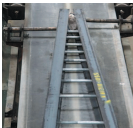
A Stobie Pole is bolted to the correct spacing and is ready for filling with concrete.
