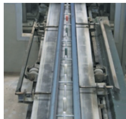
A pole is bolted to the correct spacing. The bolts also act as reinforcement rods. The plastic caps are the cores for future fixture holes that will be mounted to the pole once it is erected on site.
