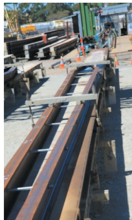
While the mechanised part of the factory is capable of producing almost every pole size, some oversized poles, such as the one shown here, are still manufactured by hand using the traditional method.
