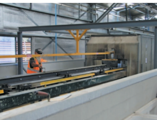
A pole that has been filled with concrete is prepared so that excess concrete can be washed off prior to curing.
