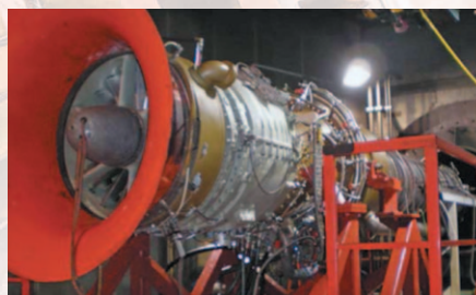
Avon 200 The modification for the upgrade can be fitted to the old Avon gas turbine during the scheduled overhaul.
