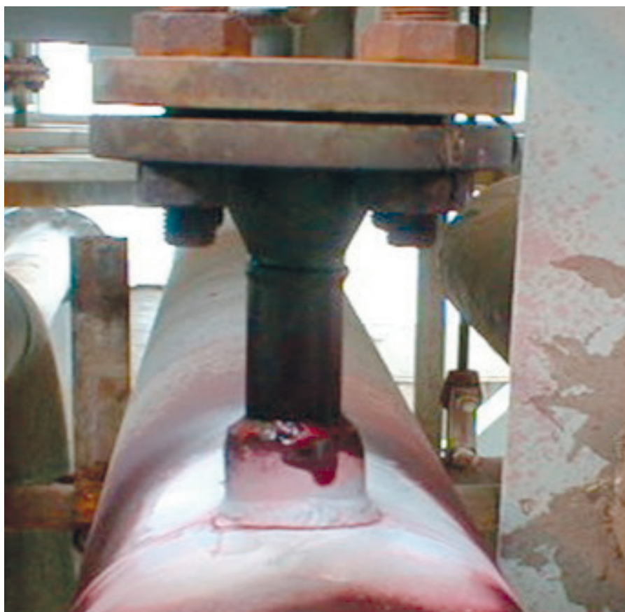
Fatigue cracking of a small bore connection caused by vibration
